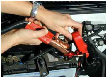
Positive to Battery Terminal
